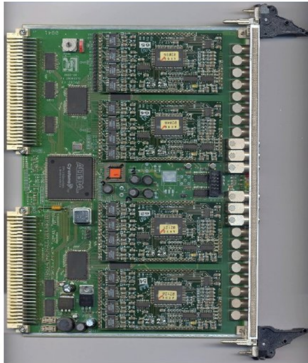
Figure 5.13: An ARS board used in the DVCS setup. These boards contain 16 channels.
