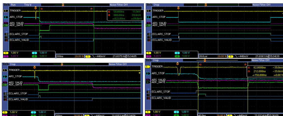
Figure 5.5: Timing measurements of the trigger module. In the four images (the horizontal lines), the yellow line is the trigger, the blue line is the ARS stop, the pink line is the ARS valid, the green line is the ADC gate. The remaining horizontal lines are the ECL signals from the lower daughter boards (with the top and last signals being copies of the ARS stop and ARS valid, while the second being the Master Or). The top-left image shows the relative timing of the ARS stop (which is seen 58 ns after the trigger) and the ARS valid (which is seen 822 ns after the trigger). The top-right image shows that the ARS stop and ARS valid go out to around 140 \mu\text{s} after the trigger is generated. The bottom-left and bottom-right images show the relative timing between the ADC gate with the trigger and the ARS stop. The ADC gate begins 60 ns after the trigger.
