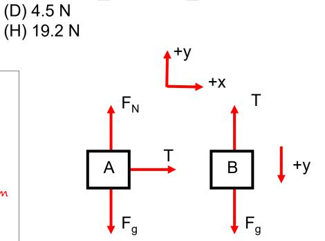
Block B of mass 1.5 kg is accelerating downward at a rate of 3.0 m/s<sup>2</sup>.
