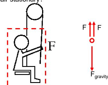
The force-multiplying power of a pulley is often referred to as its "mechanical advantage". In reality it is reduced somewhat by the pulley friction. A person who weighs 800N is sitting on a chair that weighs 10N.
