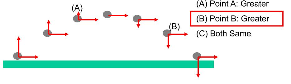
Note the symmetry. If there is no air resistance (always the case for this class), at a fixed height magnitude of velocity as it comes down is the same as when it was going up (Though the directions are different.)
