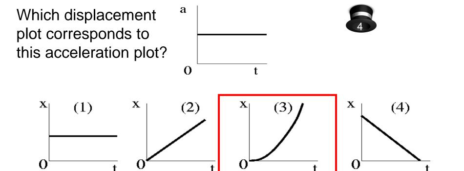
When x vs t function curves upward  $\rightarrow$  positive acceleration.
