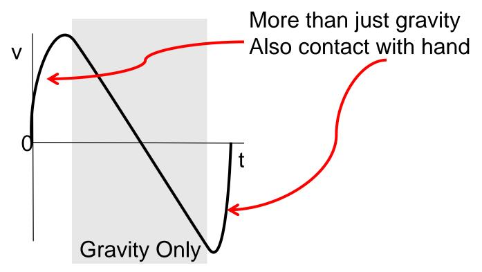
Free-fall means gravity is the only force acting on the object.
