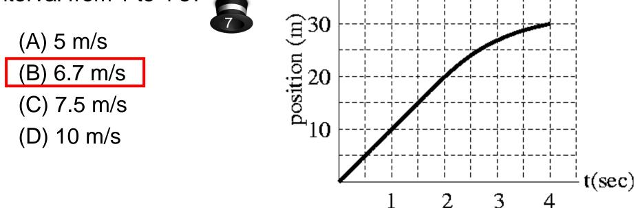
$$\overline{v} = \frac{\Delta x}{\Delta t} = \frac{x_f - x_0}{t_f - t_0} = \frac{30m - 10m}{4s - 1s} = 6.7m / s$$
