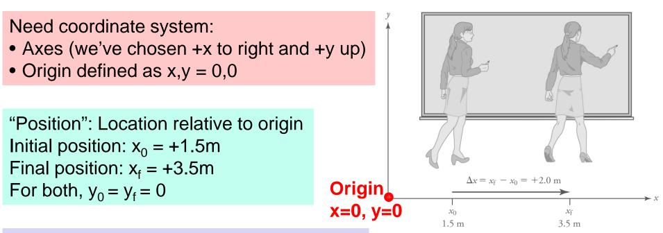
"Displacement": Change in Position  $\Delta x = x_f - x_0$ Displacement would be 2.0m to the right ( $\Delta$  = change = final - initial)
