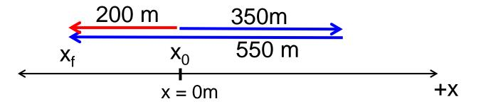
Displacement: Distance Traveled:  $\Delta x = x_f - x_0 = -200 \text{ m} = -200 \text{ m}$ (200 m to the left of the origin) Distance Traveled: 350m + 550m = 900m
