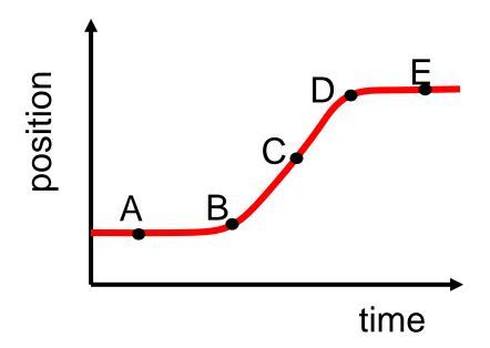
Slope represents the velocity. At Point B the slope is increasing as time increases.
