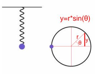
Note that  $y/r = sin(\theta)$ . So how far an oscillator is through one cycle is independent of the amplitude. I.e. the oscillation period is independent of the oscillation amplitude.
