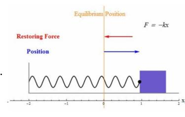
This graph represents the displacement of a mass in a mass-spring system. At which point(s) is the magnitude of the force at a maximum?
