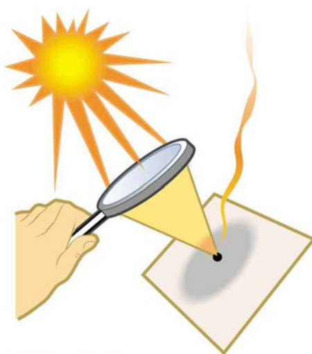
Figure 25.28 Sunlight focused by a converging magnifying glass can burn paper. Light rays from the sun are nearly parallel and cross at the focal point of the lens. The more powerful the lens, the closer to the lens the rays will cross.
