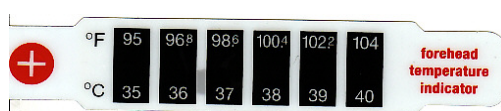
Figure 13.4 Each of the six squares on this plastic (liquid crystal) thermometer contains a film of a different heat-sensitive liquid crystal material. Below 95^{\circ}\text{F} , all six squares are black. When the plastic thermometer is exposed to temperature that increases to 95^{\circ}\text{F} , the first liquid crystal square changes color. When the temperature increases above 96.8^{\circ}\text{F} the second liquid crystal square also changes color, and so forth. (credit: Arkrishna, Wikimedia Commons)
