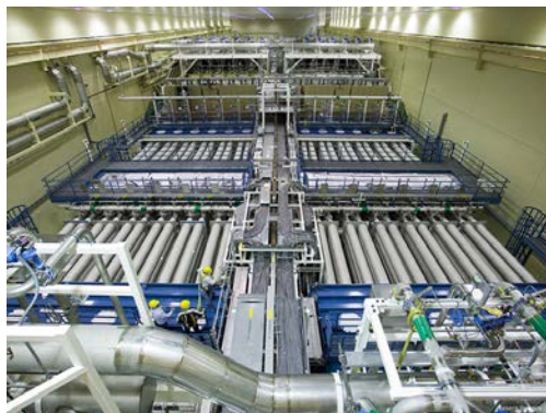
Figure 32.23 National Ignition Facility (CA). This image shows a laser bay where 192 laser beams will focus onto a small D-T target, producing fusion. (credit: Lawrence Livermore National Laboratory, Lawrence Livermore National Security, LLC, and the Department of Energy)
