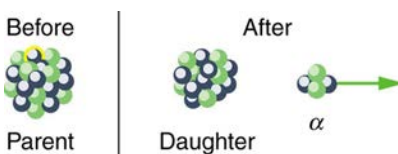
Figure 31.17 Alpha decay is the separation of a {}^4\text{He} nucleus from the parent. The daughter nucleus has two fewer protons and two fewer neutrons than the parent. Alpha decay occurs spontaneously only if the daughter and {}^4\text{He} nucleus have less total mass than the parent.
