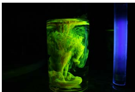
Figure 30.33 Here, fluorescent powder is added to a beaker of water. The mixture gives off a bright glow under ultraviolet light. (credit: Bricksnite, Wikimedia Commons)
