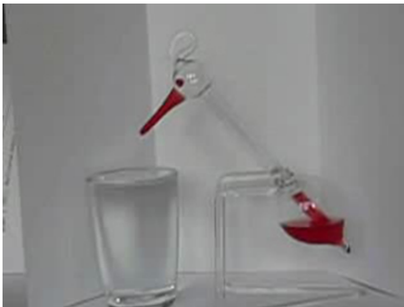
Figure 15.21 This novelty toy, known as the drinking bird, is an example of Carnot's engine. It contains methylene chloride (mixed with a dye) in the abdomen, which boils at a very low temperature—about 100^{\circ}\text{F} . To operate, one gets the bird's head wet. As the water evaporates, fluid moves up into the head, causing the bird to become top-heavy and dip forward back into the water. This cools down the methylene chloride in the head, and it moves back into the abdomen, causing the bird to become bottom heavy and tip up. Except for a very small input of energy—the original head-wetting—the bird becomes a perpetual motion machine of sorts. (credit: Arabesk.nl, Wikimedia Commons)
