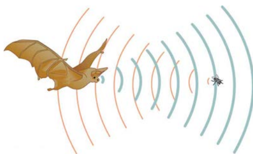
Figure 17.10 A bat uses sound echoes to find its way about and to catch prey. The time for the echo to return is directly proportional to the distance.
