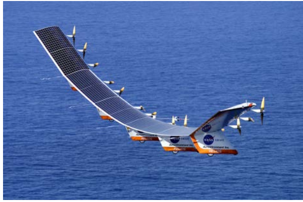
Figure 7.21 Solar energy is converted into electrical energy by solar cells, which is used to run a motor in this solar-power aircraft. (credit: NASA)
