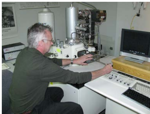
Figure 26.21 An electron microscope has the capability to image individual atoms on a material. The microscope uses vacuum technology, sophisticated detectors and state of the art image processing software. (credit: Dave Pape)
