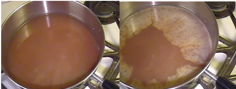
Figure 3.1: Onset of convection in a tea-milk mixture.
