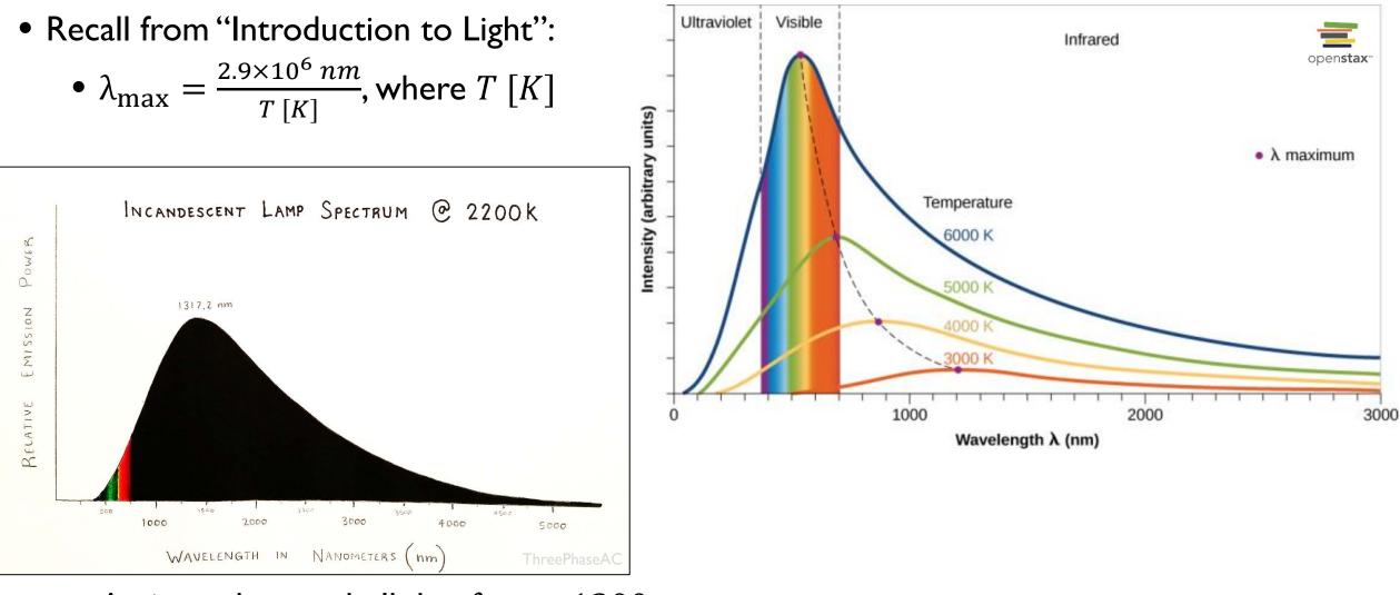
• An incandescent bulb has  $\lambda_{max} \sim 1300 nm$ So,  $T_{bulb} \approx (2.9 \times 10^6 nm)/(1300 nm) = 2200 K \sim 3500 F$
