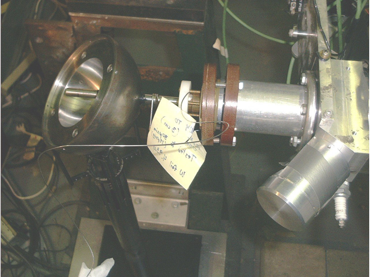
Figure II.4 Setup for the small sphere in the February 2002 experiment. The new style gas cell is shown with attachment to the beam line at the right. The water cooling coil for the cell is shown outside of the cell to the right of the sphere in this picture, near the edge of the yellow label.
