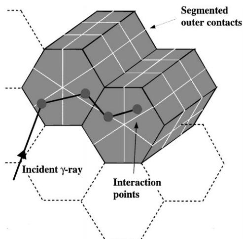
Fig. 3. Schematic view of interactions (dots) of an incident  $\gamma$ -ray in highly segmented HPGe detectors. The positions and energies of the interactions are used to reconstruct the energy and angle of the incident  $\gamma$ -ray.
